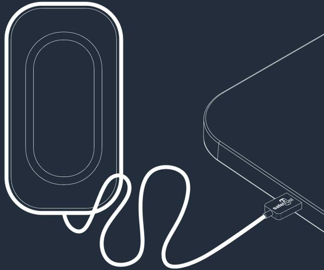
To install, simply uncoil the cord and plug the IoT Sensor USB Reader/or Programmer into your laptop or desktop computer. Within 5 seconds, the IoT Sensor will complete its "power on cycle" and be operational and ready for configuration.
