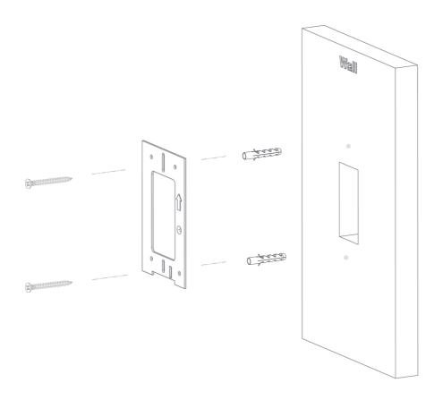
For a wall mounted installation, begin by pre-drilling your holes and insert the nylon wall plugs provided to support the weight of the reader. Once secured, you can fix the backplate to the wall using the Phillips sheetmetal screws (#6 x 1.5") provided.
