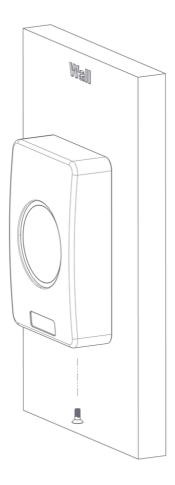
Complete the hardware installation by fixing the screw (#6-32  $\times$  .375" Phillips flat head screw) through the base of the reader.
