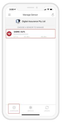
With the Manage Sensor tab open, bring the phone in range of the IoT Sensor and once visible from the App, highlight and select the "Configure" button.
