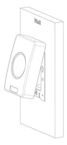
Once the backplate has been fitted and the wiring is complete, the IoT Sensor can be mounted to the wall as shown above.
