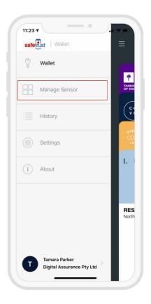
Open the Safetrust Wallet App and select the Manage Sensor tab from the navigation. Make sure your system administrator has set you up with a role that has rights to configure a sensor.
