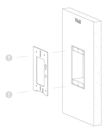
Locate the electrical box which will be recessed into the wall. You will see a top and bottom metal flange with holes which is used to secure the back plate to the wall. For this process you will need to use screws that are suitable for fixing to your specific electrical box (these are not supplied by Safetrust). Using the appropriate screws, fix the the backplate against electrical box so that it's flush.
