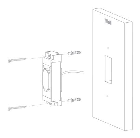
For a wall mounted installation, begin by pre-drilling your holes and insert the nylon wall plugs provided to support the weight of the reader. Once secured, you can fix the IoT Sensor to the wall using the Phillips sheetmetal screws (#6 x 1.5") provided.
