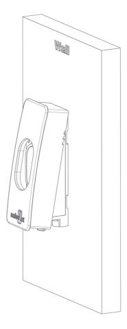
The top cover can then be fixed over the IoT Sensor as shown above.
