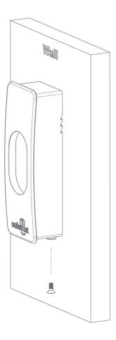
Complete the hardware installation by fixing the screw (#6-32  $\times$  .375" Phillips flat head screw) through the base of the reader.
