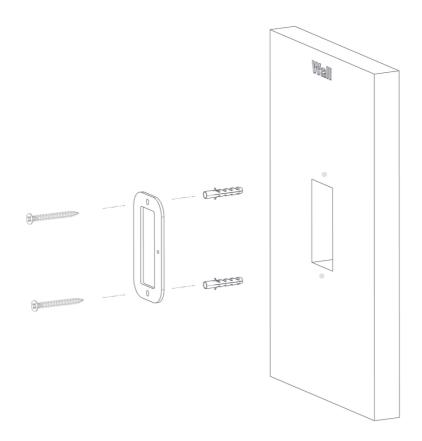
For a wall mounted installation, begin by pre-drilling your holes and insert the nylon wall plugs provided to support the weight of the reader. Once secured, you can fix the backplate to the wall using the Phillips sheetmetal screws (#6 x 1.5") provided.
