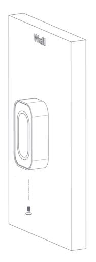
Complete the hardware installation by fixing the screw (#6-32 x .375" Phillips flat head screw) through the base of the reader.
