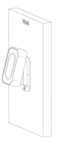
Once the backplate has been fitted and the wiring is complete, the IoT Sensor can be mounted to the wall as shown above.
