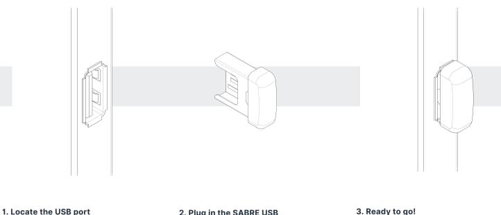
Find any spare USB port on your computer or printer to plug the SABRE USB into.
